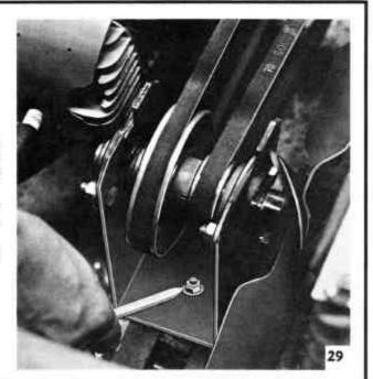
(f) Remove entire layshaft bracket, complete with belts (Fig. 30).
