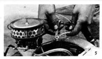
(c) Loosen clamps and detach flexible pipe connecting engine to muffler (Fig. 6).
